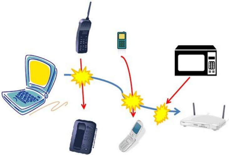
Example of devices causing interference
